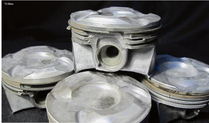
**FIGURE 3 PISTON DAMAGE OCCURRING AS THE RESULT OF LOW-SPEED PRE-IGNITION LEADING TO MEGA-KNOCK (FROM MAYER, 2016A)**
