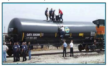
stakeholders share a commitment to safety as a top priority. Ethanol a flammable liquid is transported using a standard DOT-111A non-pressure railcar, a workhorse of the liquid transportation industry. After a few fiery accidents moving flammable liquids there has been a variety of methods to address the risks of the bulk transport of flammable liquids by rail. These efforts include issuing guidance, conducting rulemakings, participating in rail
