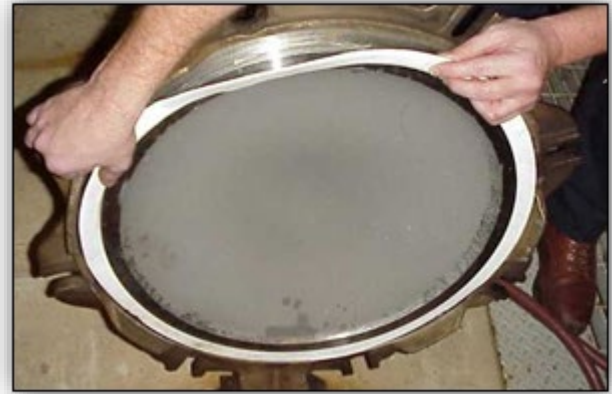
Figure 9: Installation of gasket.
