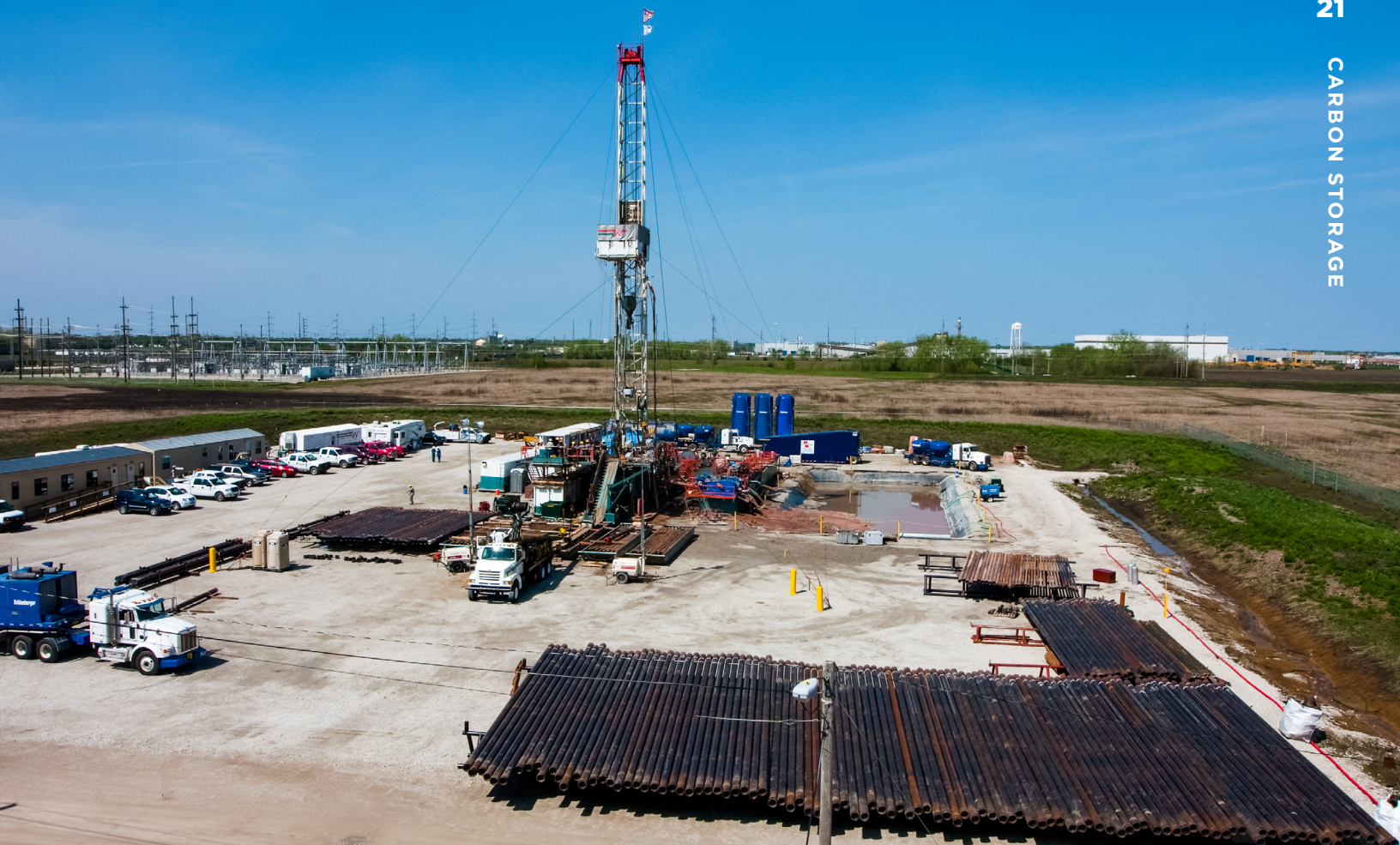
FIGURE 11. Drilling rigs like the one shown above are used across various phases of the carbon storage process. During the exploration phase, they dig exploration wells to determine storage site suitability. In the development phase, they drill the injection wells for carbon dioxide (CO 2 ) and to perform maintenance during periods of active CO 2 injection. Lastly, they are used in the decommissioning phase for operations such as well plugging and abatement procedures.
