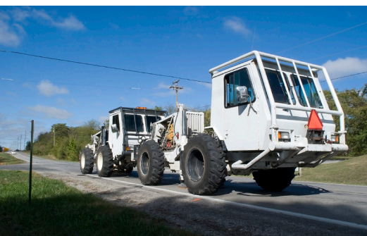
FIGURE 12. Seismic imaging is used to provide a picture of what is happening underground. By using specially equipped trucks like the one shown above to send sound waves from the surface to bounce off the underlying rocks, scientists develop a seismic map of the subsurface.
