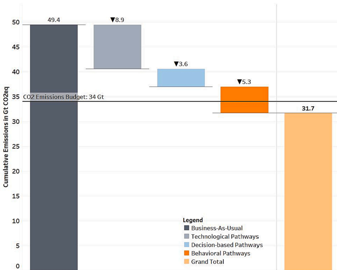
Fig. 6. Breakdown of the U.S. LDV cumulative emissions savings from 2021 through 2050 in the Conventional Road – Steady Progress Scenario (adjusted to account for 0% annual VKT growth rate) by type of pathway (technological, decisional and behavioral) with respect to the BAU Scenario). The ‘Grand Total’ column shows the cumulative (remaining) emissions of the fleet in the Steady Progress Scenario.
