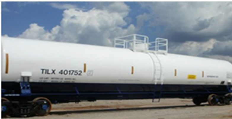
Figure 26. 21,964 gallon non-coiled, insulated car designed to operate at a 286,000 lbs. gross rail load for the transportation of carbon dioxide.
