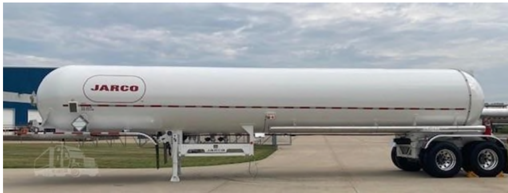
Figure 25. 10,600-gallon, 265 PSI, MC 331 Liquid Tanker
