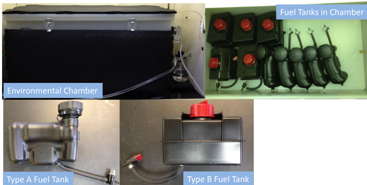
Figure 3. Photograph of fuel tanks and environmental chamber. Type A tank = Honda EVOH/LDPE, Type B tank = Tecumseh HDPE.
