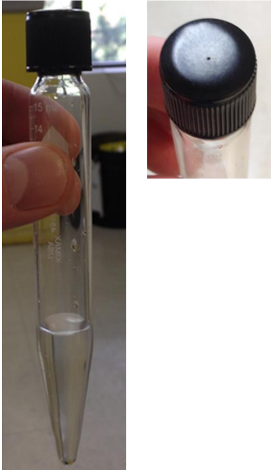
Figure 2. Test tubes, caps, and drilled hole vent.
