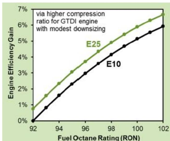
FIGURE 5 ENGINE EFFICIENCY GAINS FROM INCREASING FUEL OCTANE RATING THROUGH ETHANOL CONTENT AND COMPRESSION RATIO INCREASES FOR A GTDI ENGINE WITH MODEST DOWNSIZING.<sup>37</sup>
