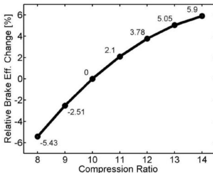
FIGURE 3 AVERAGE RELATIVE BRAKE EFFICIENCY CHANGE VERSUS COMPRESSION RATIO FOR ALL DATA SETS WITH RELATIVE VALUES FROM UNIT CHANGES IN COMPRESSION RATIO LABELLED.<sup>23</sup>
