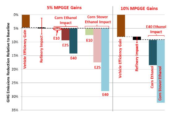
FIGURE 6 WTW GHG EMISSIONS REDUCTIONS IN VEHICLES FUELD BY HOFS WITH DIFFERENT ETHANOL BLENDING LEVELS RELATIVE TO REGULAR GASOLINE (E10) BASELINE VEHICLES.<sup>41</sup>
