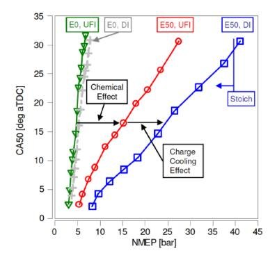
FIGURE 4 SEPARATION OF CHEMICAL OCTANE AND CHAGE COOLING EFFECTS ON KNOCK LIMIT FOR B88E5—R105 AT 10:1 CR AND 1500 RPM.
