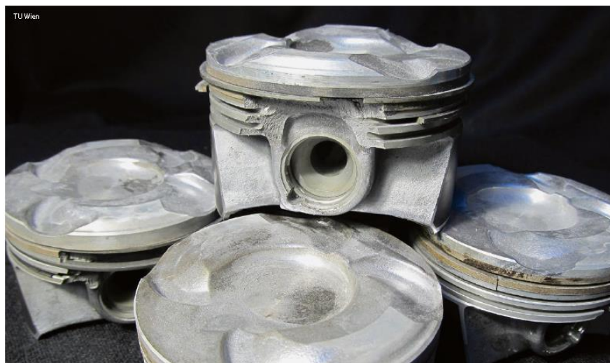
FIGURE 3 PISTON DAMAGE OCCURRING AS THE RESULT OF LOW-SPEED PRE-IGNITION LEADING TO MEGA-KNOCK (FROM MAYER, 2016A)
